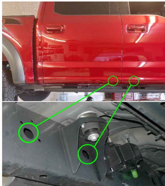
Figure 14- Raptor-203 Install Location
